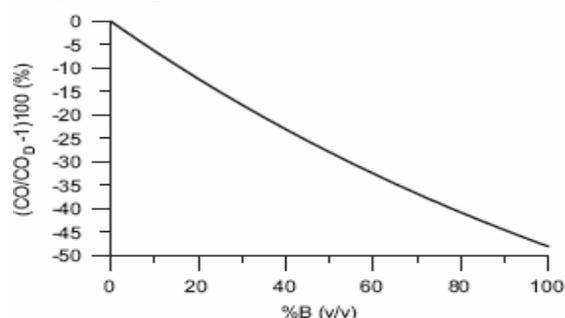
**Figure 4.** Mean reduction in CO emissions as the biodiesel content increases (trend obtained from Ref. [24] for heavy-duty engines with no EGR).
