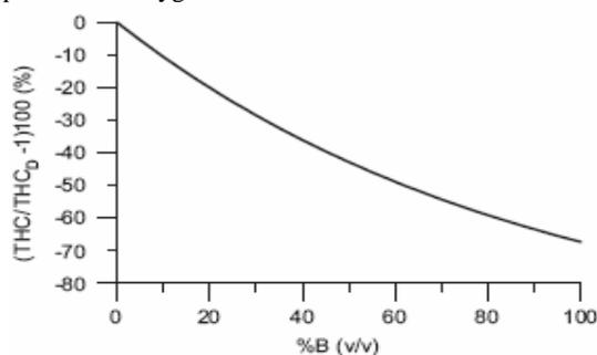
**Figure 3.** Mean reduction in Total Hydro Carbon (THC) emissions as the biodiesel content increases (trend obtained from Ref. [24] for heavy-duty engines with no EGR).
