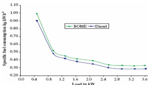
**Figure 2.** Variation of specific fuel consumption in kg/kWh with applied load (courtesy S.J. Deshmukh and L.B. Bhuyar [15]).
