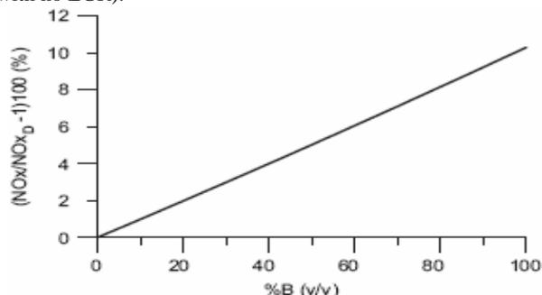
**Figure 5.** Mean reduction in NO<sub>x</sub> emissions as the biodiesel content increases (trend obtained from Ref. [24] for heavy-duty engines with no EGR).
