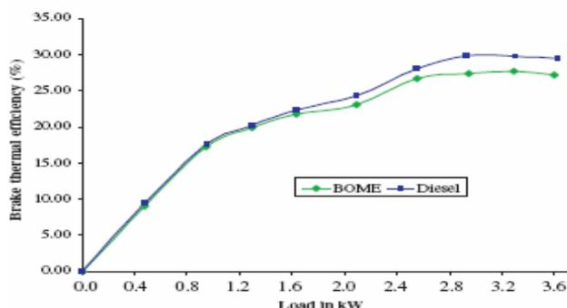
**Figure 1.** Variation of brake thermal efficiency with load (courtesy S.J. Deshmukh and L.B. Bhuyar [15]).
